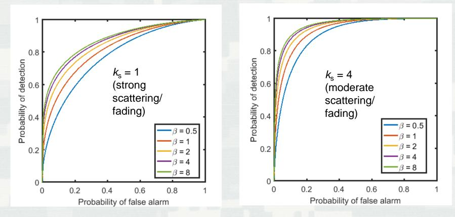
Receiver operating characteristic (ROC) curves corresponding to a gamma-distributed signal with the specified shape factor and gamma-distributed noise with  $k_n = 4$ . The signal-to-noise ratio (SNR) is 2, and the hyperparameter  $\beta$  is varied as shown in the legend. (The hyperparameter  $\alpha$  is set to  $k\beta$ +1, so that the mean signal power is 1.)
