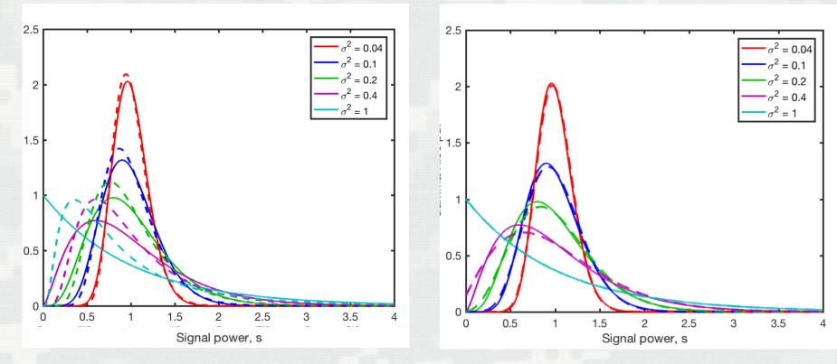
Gamma (solid lines) and log-normal (dashed lines) pdfs for various values of the variance normalized by the squared mean. For weak scattering (which is the intended application of the log-normal distribution), the pdfs are nearly identical. Gamma (solid lines) and Rice (dashed lines) pdfs for various values of the variance normalized by the squared mean. For both strong and weak scattering, the pdfs are nearly identical. At intermediate cases, there are subtle differences.
