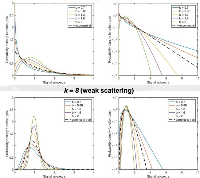
The parameter *b* is seen to control the "tails" of the distribution. As *b* decreases, the pdfs change from a normal-like appearance to having tails exceeding the gamma distribution for the corresponding value of *k*.
