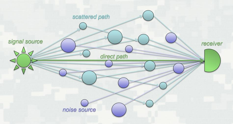
The received signal consists of the signal of interest, which propagates along and direct path and multiple randomly scattered paths, and noise from multiple, random sources.
