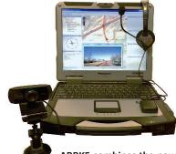
ARRK5 combines the power of an interactive touch screen computer with a headset, GPS, and a high-resolution digital camera.
