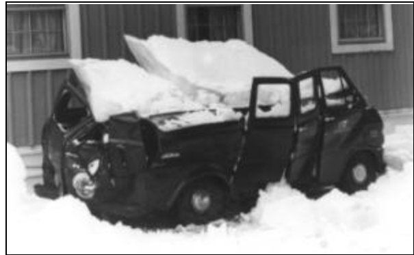
Figure 6. Vehicle damaged by snow and ice that fell from a roof.
