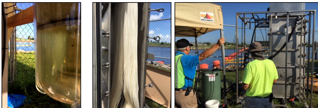
Figure 2-9. Testing of stacked disk filter (left) and ZeeWeed hollow fiber membranes (middle, right) for algae removal at the Moore Haven demonstration site.
