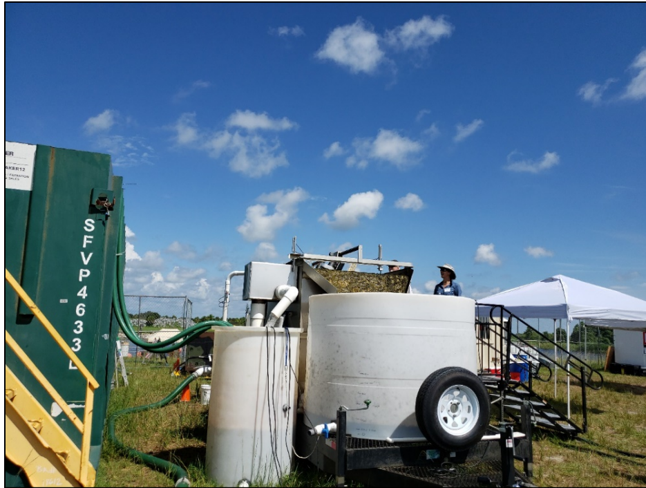
Figure A-14. Skimming of the separated algae into a collection tank.
