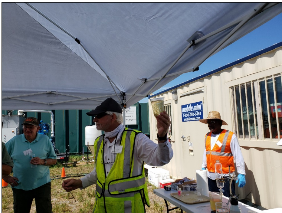
Figure A-7. Visible coagulation of algal cells within 2 minutes of adding reagents.
