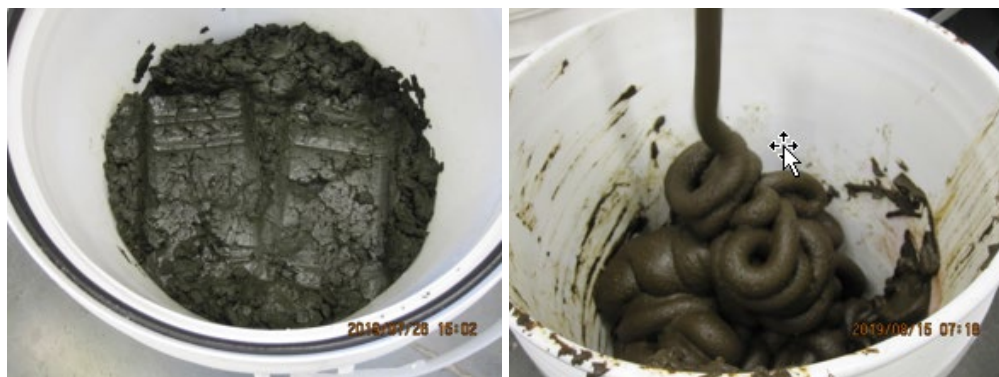
Figure 2-12. Preparation of algal biomass for hydrothermal liquefaction (HTL) testing at the Pacific Northwest National Laboratory (PNNL).
