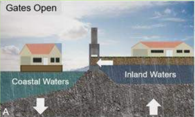
Gravity draining inland flood water to the coast
