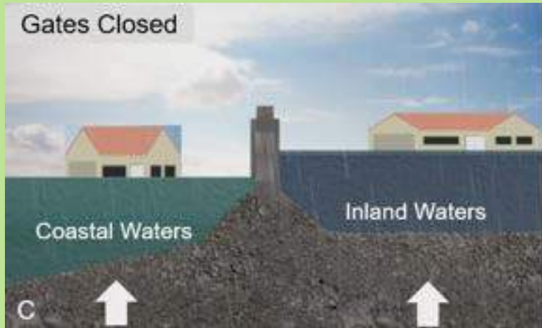
Gates closed due to increased coastal waters, which results in increased inland flood waters, combined with high groundwater levels
