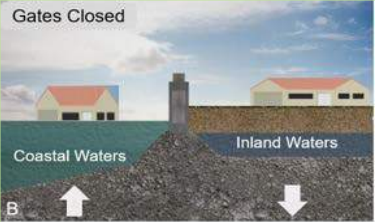
Gates closed due to increased coastal waters, stopping saltwater intrusion
