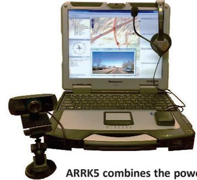
**ARRK5 combines the power of an interactive touch screen computer with a headset, GPS, and a high-resolution digital camera.**
